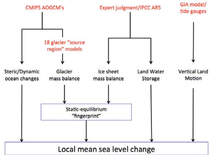
**Figure 2:** Schematic illustration of the sources of information (red) and physical processes (black) included in the mean sea level projections
